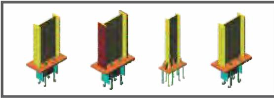
SHEAR CONNECTION - BEAM TO COLUMN
